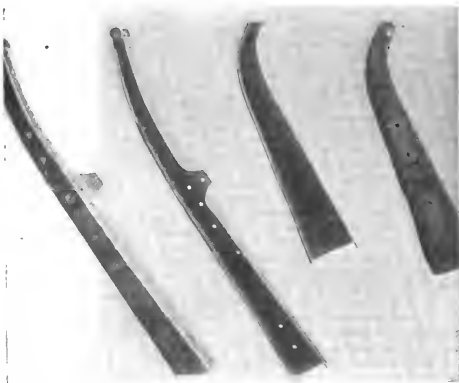
FIG. 6.—Four expensive breaks, all on cars of the same high-priced make and all due to the same cause—improper material.
